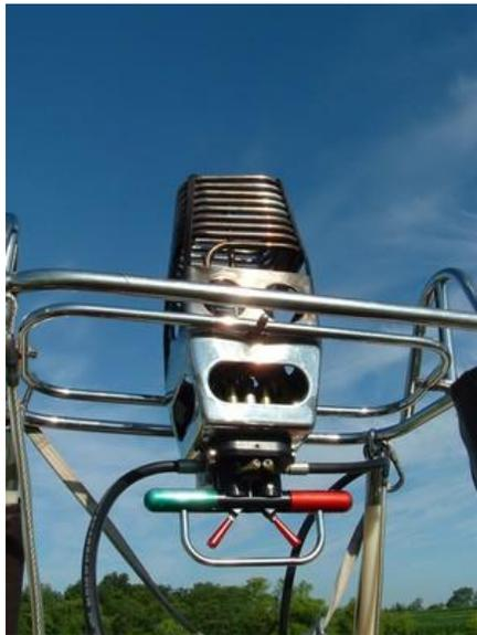
Single Burner and Burner Frame
